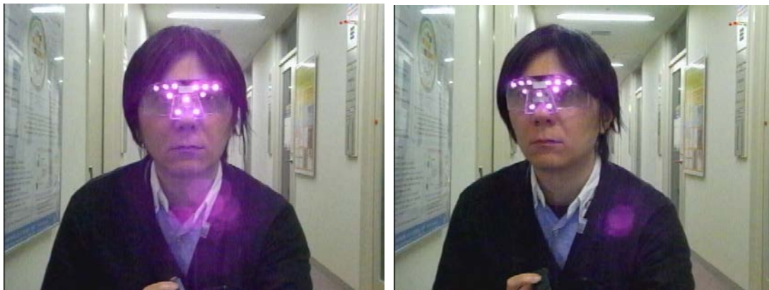
(b) Near infrared LED lit (detection failed)
