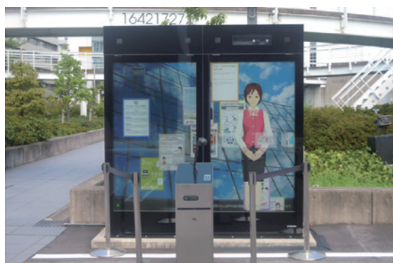
Photo 1: A digital signage constructed for navigation of the campus of Nagoya Institute of Technology. The digital signage has a speech recognition/speech synthesis/CG system. A CG character communicates interactively with visitors through speech. The speech synthesis system "HTS" and the speech recognition engine "Julius" that are used in this system are released as open-source software named "MMDAgent."
