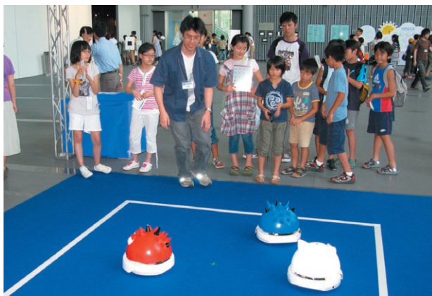
Demonstration of ultrasonic positional recognition (at Interactive Tokyo 2008).
