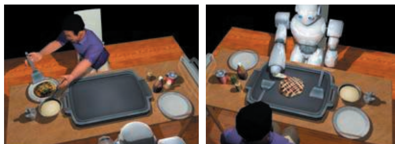
Fig. 2 “Cooking Okonomiyaki” Collaborative Task in the SIGVerse Left: An avatar operated by a user moves the okonomiyaki to a plate. During this process, the robot observes the behaviors of the avatar and decides a suitable support behavior that can be done parallel. Right: The user hardly operated the avatar at all, so the robot is cooking the okonomiyaki by itself. In this way, it is possible to create a program that determines behaviors of the intelligent robot by confirming how the robot behaves in response to user behavior.
