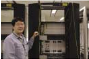
Optical cross-connects (OXC) are devices for switching circuit connections. There are two kinds of cross-connects: electronic cross-connects that once convert the optical signals to electrical signals, and optical cross-connects that can switch the optical signal without any conversion.
