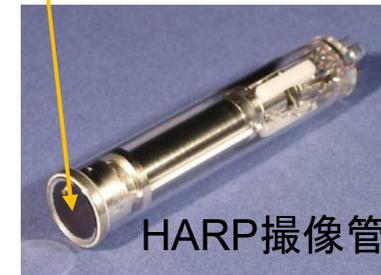
HARP: High-gain Avalanche Rushing amorphous Photoconductor
