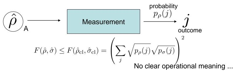
The equality is always achieved by the orthogonal measurement on a basis "diagonalizing  $\sqrt{\hat{\rho}}/\sqrt{\hat{\sigma}}$ ."
