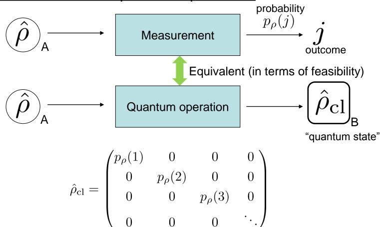
Any measurement has a description in terms of a quantum operation.
