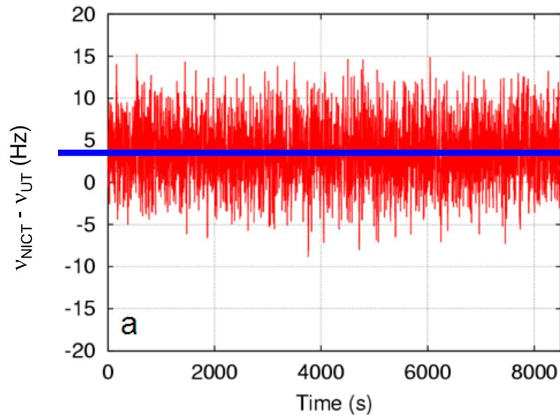
A Hz-level frequency difference is clearly visible over the time scale of minutes
