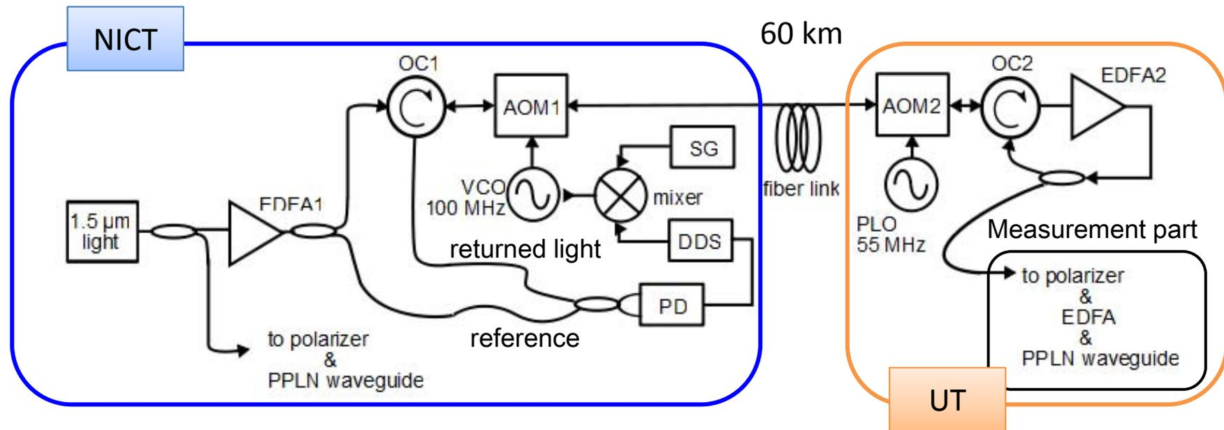
Transfer system based on a fiber interferometer
