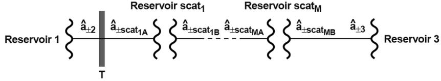
Figure 5.17: A two-port conductor with an elastic scatterer having a finite transmission probability,  $T$ .  $M$  purely inelastic scattering voltage probes are added after the scatterer.
