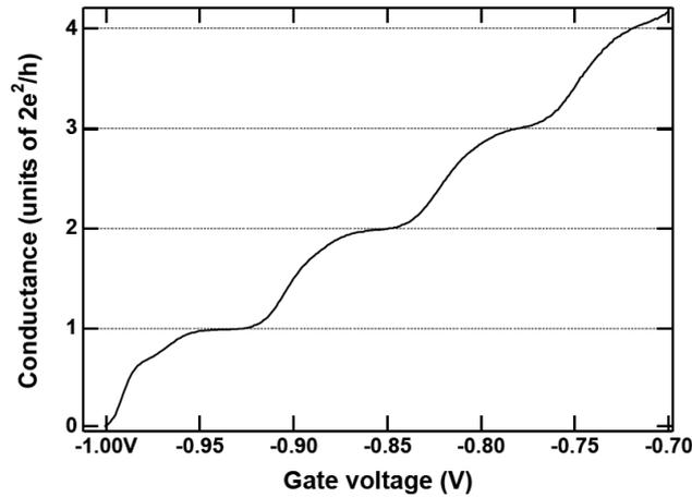
Figure 5.4: The conductance of a QPC vs. the gate voltage. The conductance is quantized in units of  $2e^2/h$ . At each plateau, all electrons injected into the transmission modes without reflection contribute to the conductance. At each step, the transmission probability of the highest transverse mode transitions from zero to unity.
