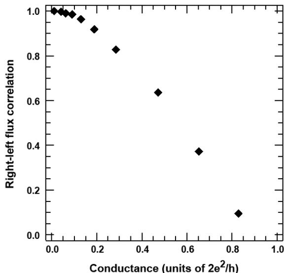
Figure 5.15: The correlation between right and left moving electrons vs. the conductance. The correlation is taken near the two-port conductor's center, and it approaches unity as elastic scattering increases.
