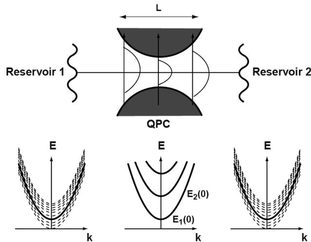
Figure 5.2: A schematic of a quantum point contact (QPC) of nominal length  $L$ , connected to large electron reservoirs. The first transverse mode propagates through the point contact. Because of the small dimension, the discrete modes,  $E_j(0)$  are well separated. In contrast, in the reservoirs, a large density of modes exists, usually one of which is mode-matched to the QPC.
