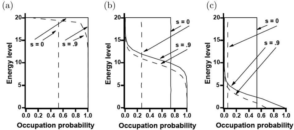
Figure 5.16: Electron energy vs. electron occupation at three different positions in the two-port conductor: (a) left, (b) center, (c) right. If the conditional probability for inelastic scattering,  $s$ , is zero, then the electrons are equally distributed in energy in both the right moving (solid line) and left moving (dashed line) directions. As  $s$  increases to .9, the lower energy states become more fully occupied, while the high energy states become unoccupied.
