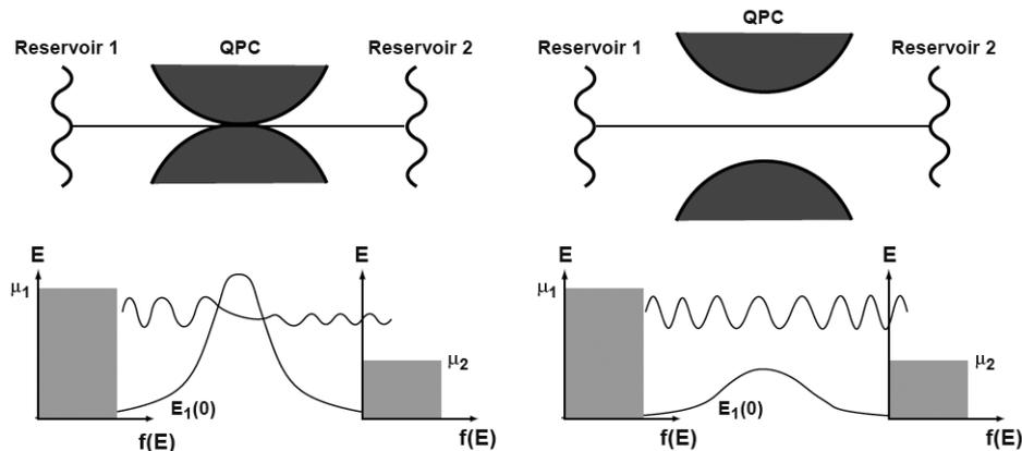
Figure 5.3: (a) QPC near pinchoff. The plane wave electron decays evanescently through the barrier, giving only a small transmission. (b) Open QPC. The subband level is now below the Fermi level so that all electrons can be transmitted with unity probability.
