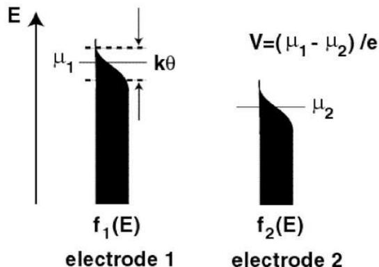
Figure 5.6: One-dimensional mesoscopic conductor at thermal equilibrium.
