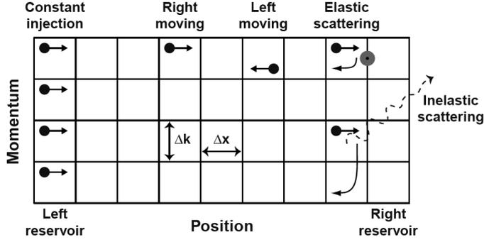
Figure 5.13: Electron phase space in the conductor. The phase space is partitioned into right and left moving electron cells of width  $\Delta x$  by  $\Delta k$ . Elastic scattering reverses the momentum while inelastic scattering also causes a loss in energy.
