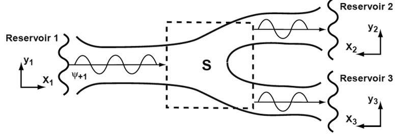
Figure 5.7: Coherent scattering model. A scattering matrix,  $s$  couples the plane wave state incident from one reservoir, e. g.  $\psi_{+1}$ , with outgoing plane waves in other reservoirs.
