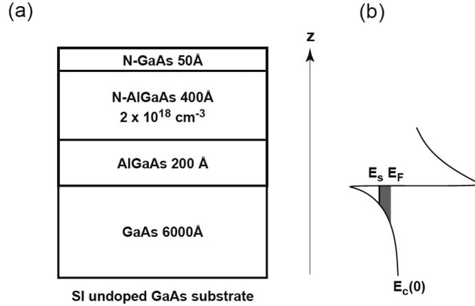
Figure 5.1: (a) The epitaxial structure of a GaAs-2DEG. (b) Conduction band energy diagram near the interface between the non-doped GaAs and AlGaAs. A two dimensional electron gas forms in the triangular well.
