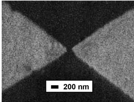
Figure 5.10: SEM photograph of one of the fabricated quantum point contacts (QPC).
