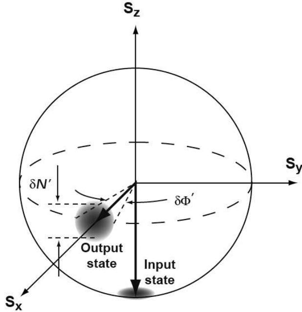
Figure 5.9: Bloch sphere diagram of the input and output spin states of the 50-50 beam splitter. The input state exhibits no number difference noise,  $\delta \mathcal{N} = 0$ , but has an indeterminate phase. The output state is a coherent spin-state with Poissonian fluctuations in both number ( $\delta \mathcal{N}'$ ) and phase ( $\delta \Phi'$ ) difference.
