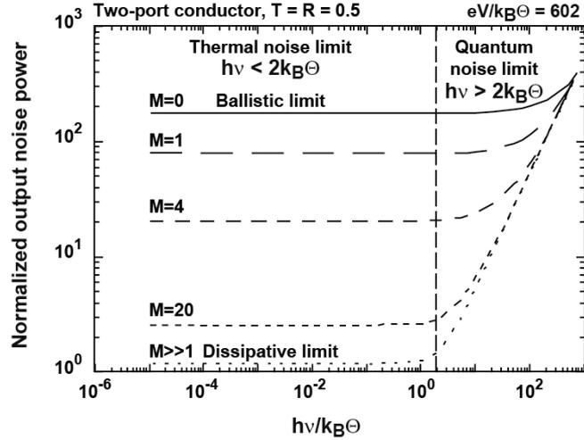
Figure 5.19: The current noise (normalized to the Johnson thermal noise with a conductance of  $TG_Q/(TM + 1)$ ) for a two-terminal device with elastic transmission  $T = 0.5$  vs. the frequency normalized by the thermal frequency. The transport noise is again suppressed to the generalized Johnson-Nyquist noise limit by increasing  $M$ .
