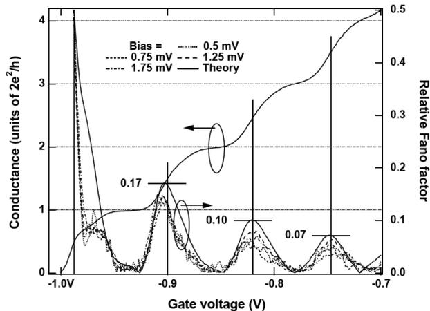
Figure 5.11: The noise power normalized by the noise power at  $T = 1/2$  vs. the gate voltage. When renormalized in this fashion, the experimental curves show reasonable agreement with theory.
