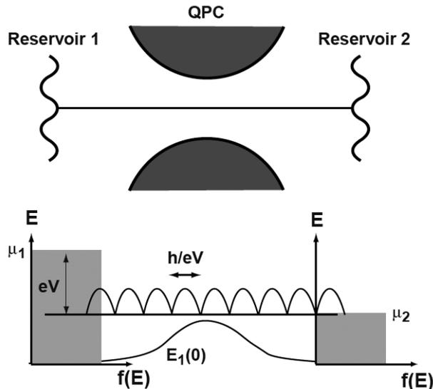
Figure 5.5: The wave packet picture of ballistic transport. An energy bias of  $eV$  injects wave packets of nominal time width  $h/eV$  into the QPC. Because of the zero temperature Fermi-Dirac distribution, the injection is quiet.
