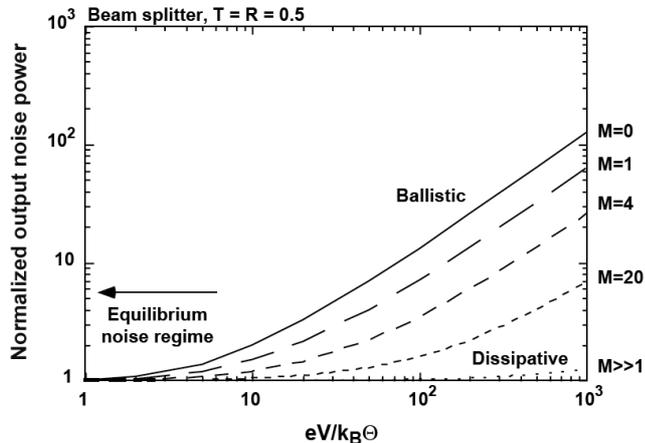
Figure 5.18: The current noise at 1 kHz (normalized to the generalized Johnson-Nyquist noise with a conductance of  $G_Q/(M + 1)$ ) vs. the voltage bias normalized by the thermal voltage,  $k_B\Theta/e$ . As inelastic scattering increases (increasing  $M$ ), the transport noise is suppressed to the generalized Johnson-Nyquist noise limit.
