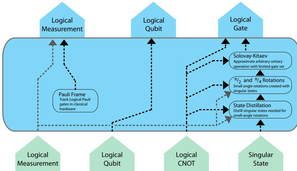
**Figure 8.** Organization of processes in the Logical layer. Logical qubits from Layer 3 are unaltered, but faulty singular states are distilled into high-fidelity states  $|Y\rangle = \frac{1}{\sqrt{2}}(|0\rangle + i|1\rangle)$  and  $|A\rangle = \frac{1}{\sqrt{2}}(|0\rangle + e^{i\frac{\pi}{4}}|1\rangle)$ . The distilled states are used to create arbitrary gates with the Solovay-Kitaev algorithm.
