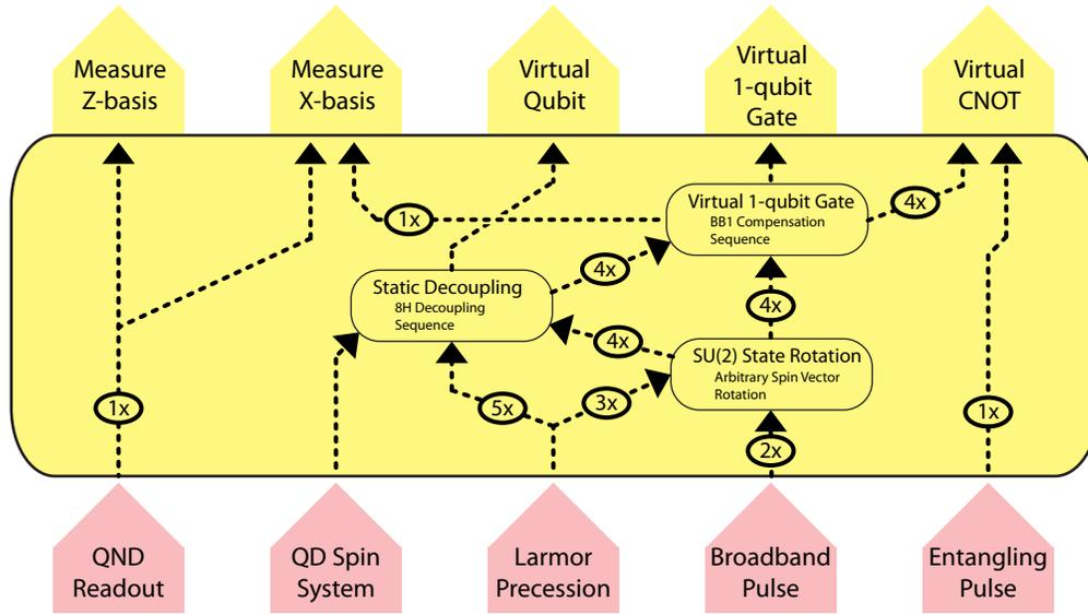
**Figure 5.** The mechanics of the virtualization layer. The outputs of Layer 1 are combined in controlled sequences to produce virtual qubits and gates. Arrows indicate how the output of one process is used by another process. The circled numbers indicate the quantity of a certain resource being used.
