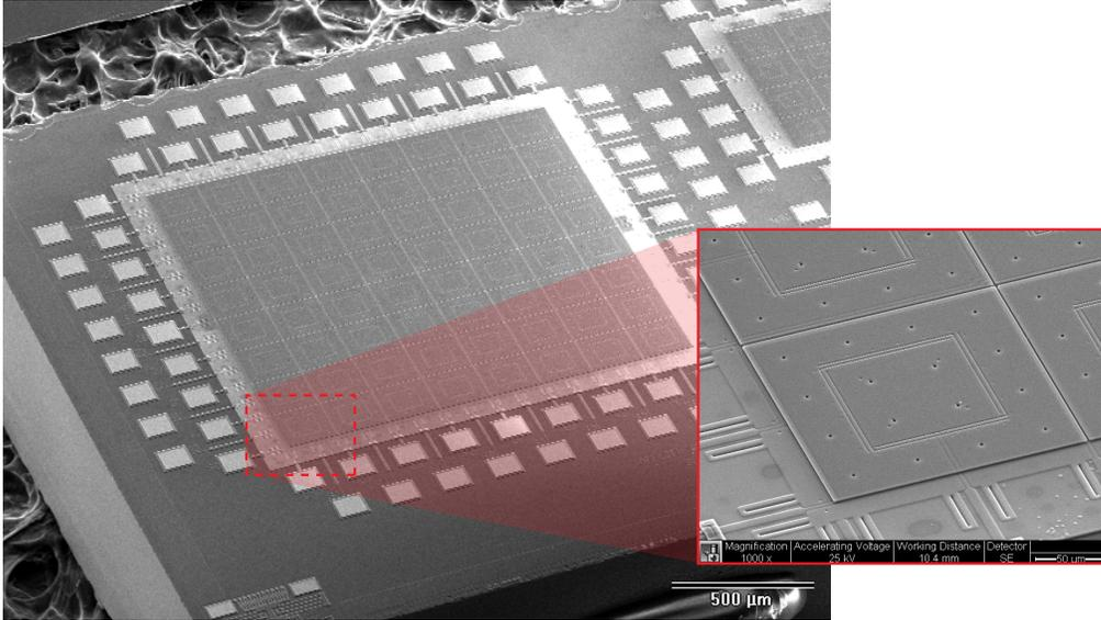
**Figure 4.** SEM image of an array of micromirrors. This image is an experimental sample of vertically actuated mirrors, whereas the MEMS array in QuDOS would require smaller size mirrors with tilting actuation at very high speeds. The inset image shows a magnified view of a single mirror.
