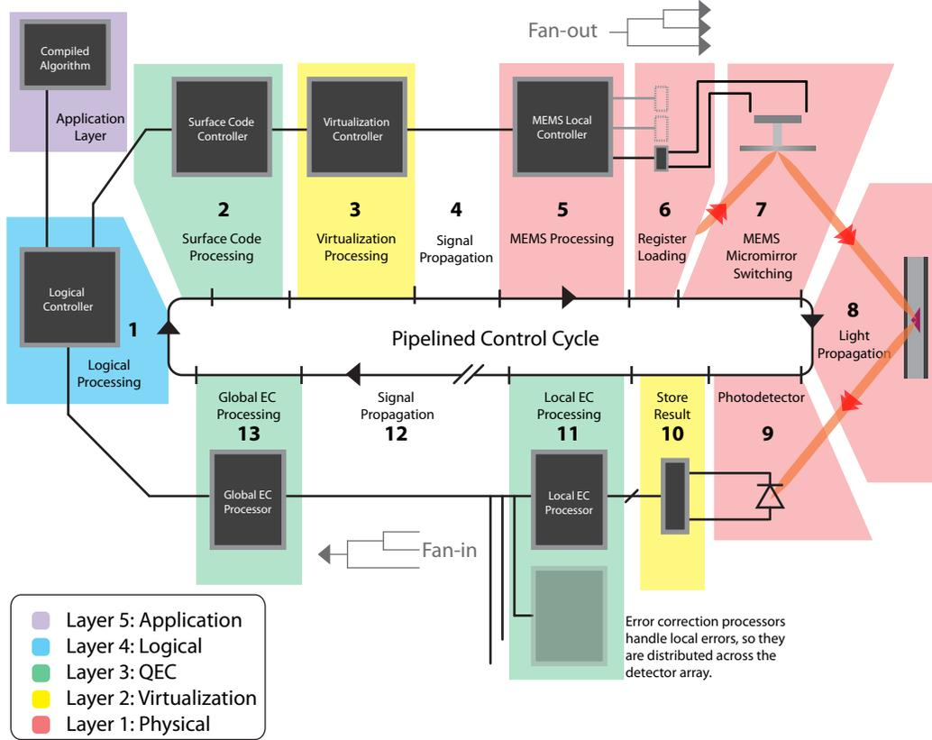
**Figure 10.** Primary control cycle of QuDOS. Though presented as a sequence of steps, each layer issues multiple commands to the layer below, and operations are pipelined. Each of the numbered steps represents a process whose time duration must be precisely determined in order for the architecture to function efficiently. Steps 4 and 12 indicate significant delays in the propagation of a control or readout signal.
