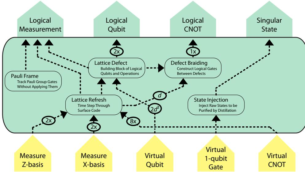
**Figure 7.** Process translation in Layer 3. A surface code is constructed with virtual qubits and gates, ultimately yielding logical qubits and operations. The arrows in yellow along the bottom are outputs of Layer 2, whereas the green arrows at the top are the outputs of Layer 3. Small dashed arrows indicate that the output of one process is used by another process. The circled number is the quantity of the corresponding resource which is used.
