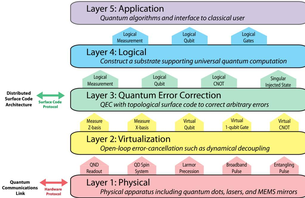
**Figure 1.** Layered control stack which forms the framework of a quantum computer architecture. Vertical arrows indicate services provided to a higher layer. Arrows on the left margin indicate that communication protocols are necessary to connect multiple quantum information devices, but this topic is outside the scope of this work.
