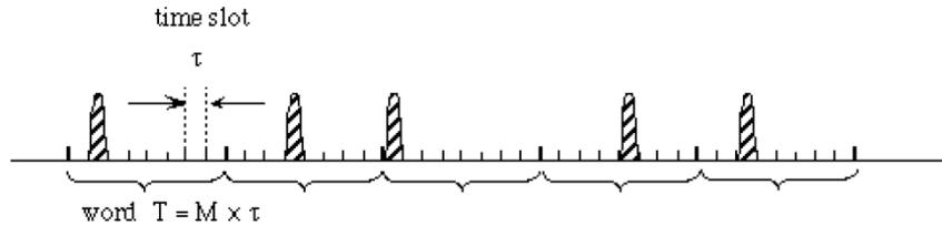
Figure 12.16: A pulse-position-modulation (PPM) signal.
