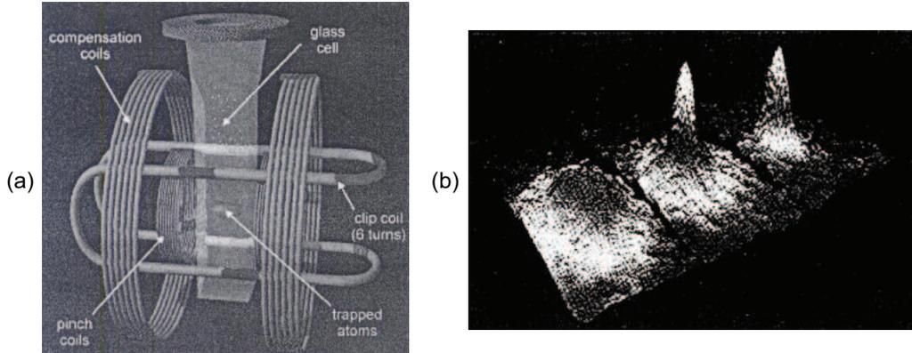
Figure 1.2: (a) A magnetic trap used for atomic BEC experiments. (b) Momentum distributions of rubidium atoms which feature a BEC phase transition [1].
