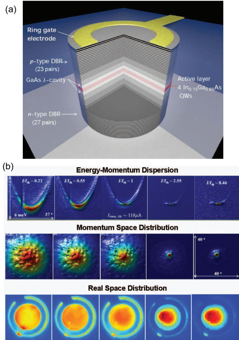
Figure 1.3: (a) A current injection type semiconductor planar microcavity with multiple quantum wells in a one-wavelength cavity, which is sandwiched by two  $p$ -type and  $n$ -type distributed Bragg reflectors. (b) Evolution of the energy-momentum dispersion relation, the momentum space distribution and the real space distribution of the exciton-polaritons across the exciton-polariton BEC phase transition.
