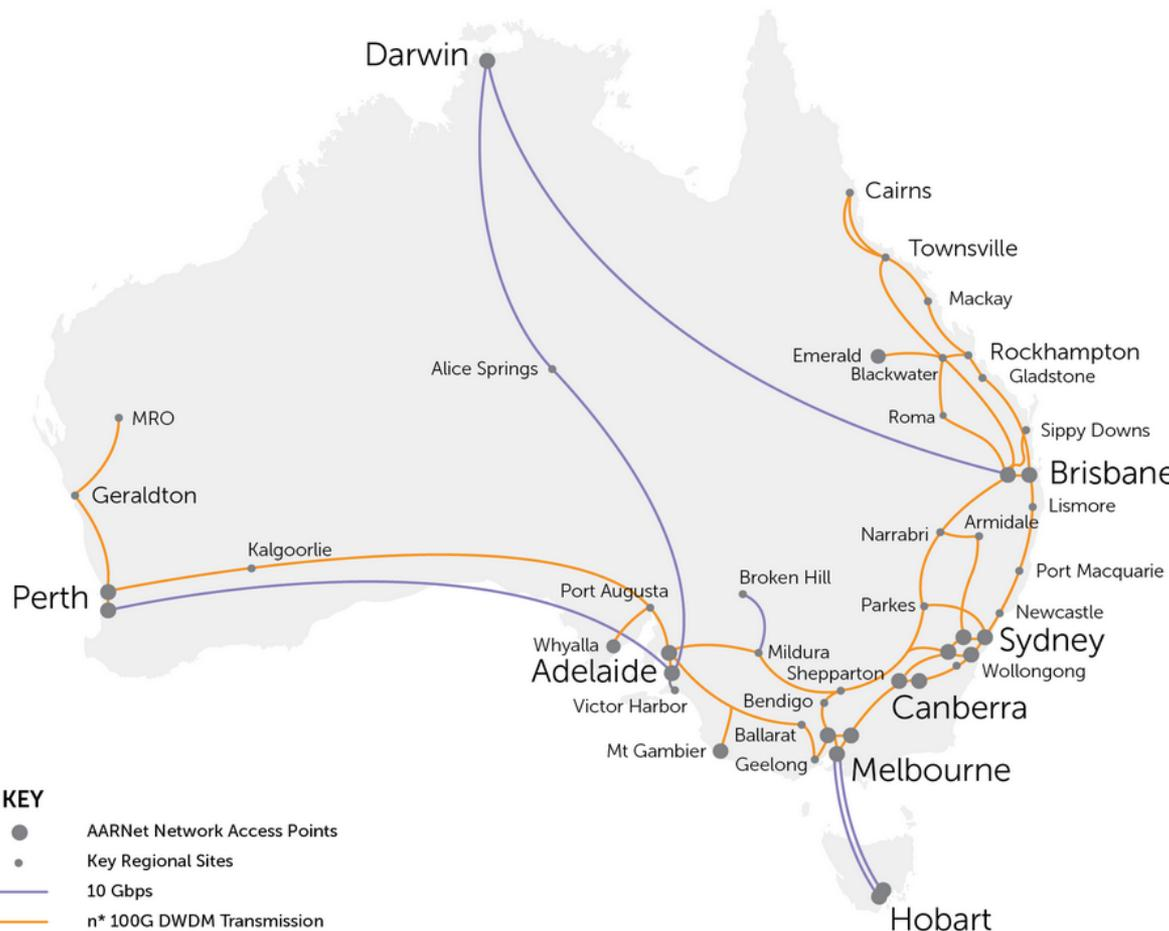
Cisco and Australia's Academic and Research Network (AARNet) have successfully demonstrated 600 Gbps on the AARNet production network using Cisco Network Convergence System (NCS) 1004. This groundbreaking terrestrial trial is a first for Australia and proves the future scalability of the AARNet network.
