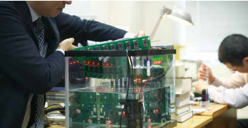
The Cooling Test for Submerging an In-water Computer and Fault-diagnosis Test Boards in Water.
