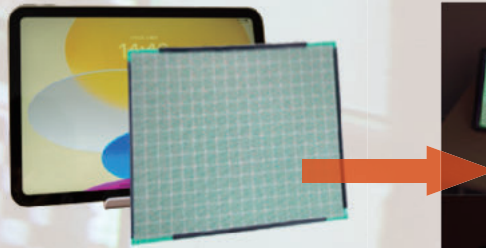
Pinhole array (simple 3D display) small Small prototype of our simple 3D display with a pinhole array for demo: A circuit board acting as pinholes is attached to a tablet to reproduce a light field. Horizontal and vertical parallax is supported. The light field image passes through the pinholes
