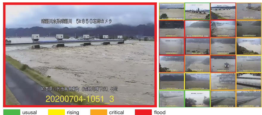
Fig.: Automatic recognition of flooding images based on deep learning (Kuma River water system). Live camera images are analyzed in real time using deep learning, and flood conditions are displayed in different colors.
