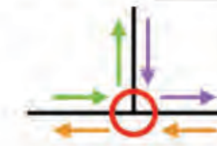
Figure 4: Loop constraints can be enforced locally at each junction. The room types must be the same for each pair of walls marked with the same color.
