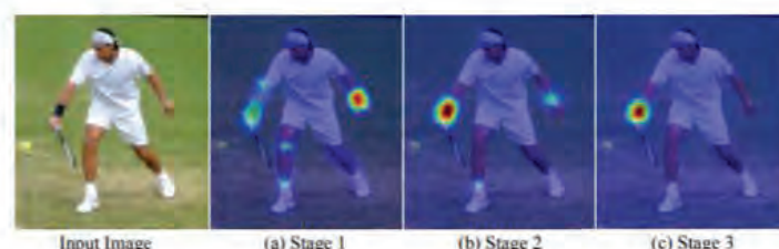
Figure 1: A Convolutional Pose Machine consists of a sequence of predictors trained to make dense predictions at each image location. Here we show the increasingly refined estimates for the location of the right elbow in each stage of the sequence. (a) Predicting from local evidence often causes confusion. (b) Multi-part context helps resolve ambiguity. (c) Additional iterations help converge to a certain solution.
