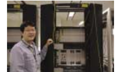
Optical cross-connects (OXC) are devices for switching circuit connections. There are two kinds of cross-connects: electronic cross-connects that once convert the optical signals to electrical signals, and optical cross-connects that can switch the optical signal without any conversion.
