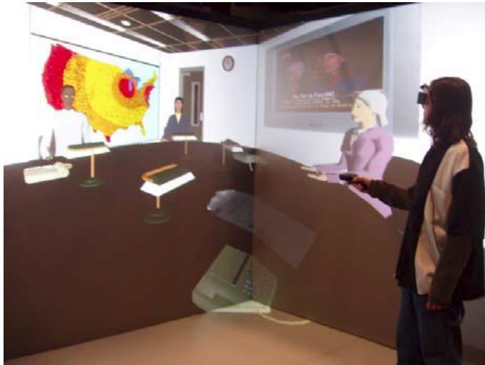
Figure 2: A user participating in Crisis Communication. The training system uses four screens and stereoscopic glasses to improve immersion.
