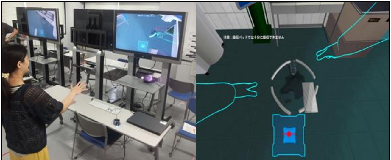
Figure 6: The Kinect control interface in Bio-Safety Lab. A user is standing in front of the Kinect device and controlling the avatar’s actions (left). The user can see his/her position inside the blue square in the bottom part of the screen, represented by a red mark (right). The inner blue square represents the area where the user can move without move the avatar. The outer square is the area in where the user has to move for moving the avatar across the room. Outside of the square, user’s movements are not detected.
