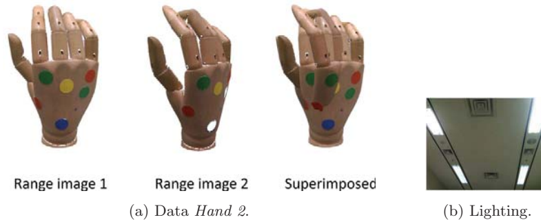
Figure 5.33: Initial estimates of registration for the data Hand 2 .
