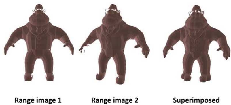
Figure 5.26: The input range images with initial estimate of registration for the scenario 2.
