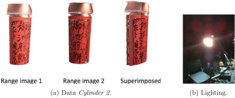
Figure 5.39: Initial estimates of registration for the data Cylinder 2 .
